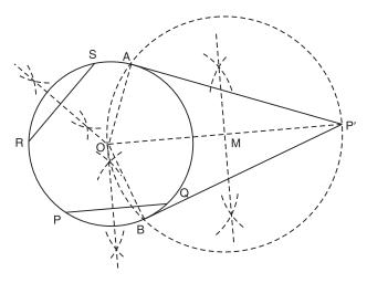
VII. Join P'A and P'B. Thus, P'A and P'B are the required two tangents.
