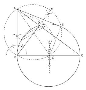
Q. 7. Draw a circle with the help of a bangle. Take a point outside the circle. Construct the pair of tangents from this point to the circle. [CBSE 2012]
