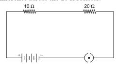
3. Find the net current flowing through the following electric circuit:
