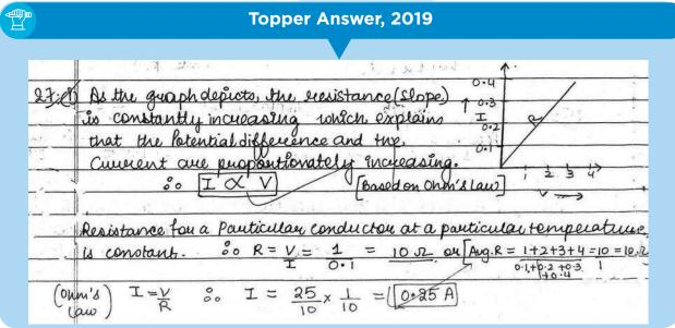
2. While studying the dependence of potential difference (V) across a resistor on the current (I) passing through it, in order to determine the resistance of the resistor, a student took 5 readings for different values of current and plotted a graph between V and I. He got a straight line graph passing through the origin. What does the straight line signify? Write the method of determining resistance of the resistor using this graph.
