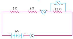
What would be the readings of the ammeter and the voltmeter when key is closed? Give reason to justify your answer.
