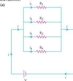
Let there be n resistance, each of value  $R_1$ ,  $R_2$ ....  $R_n$  respectively connected in parallel to a battery of voltage V.
